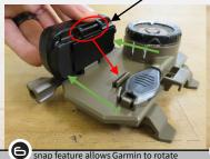
up providing access to the battery door and USB port
