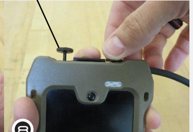
8 hold down middle of cable while tightening screws
