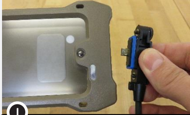
1 remove Quick Disconnect Cable Assembly prior to inserting **critical step**
