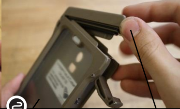
2 open door latch to release door
