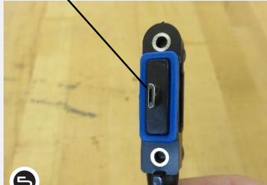
5 inspect cable to ensure that the seal is clean and still attached
