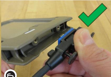
6 connect micro USB with cable facing toward the left side of the device/case
