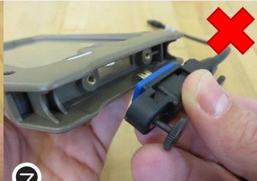
7 do not connect with the cable facing to the right
